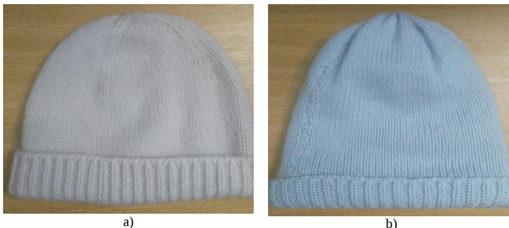
Fig. 5: The product obtained by a) full knitting b) the classic knitting method
